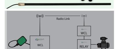
When the float switch in the water tank hits the low level setpoint, an on command is sent to the pump via radio. When the water tank level hits the high setpoint, a stop command is sent to the pump via radio
